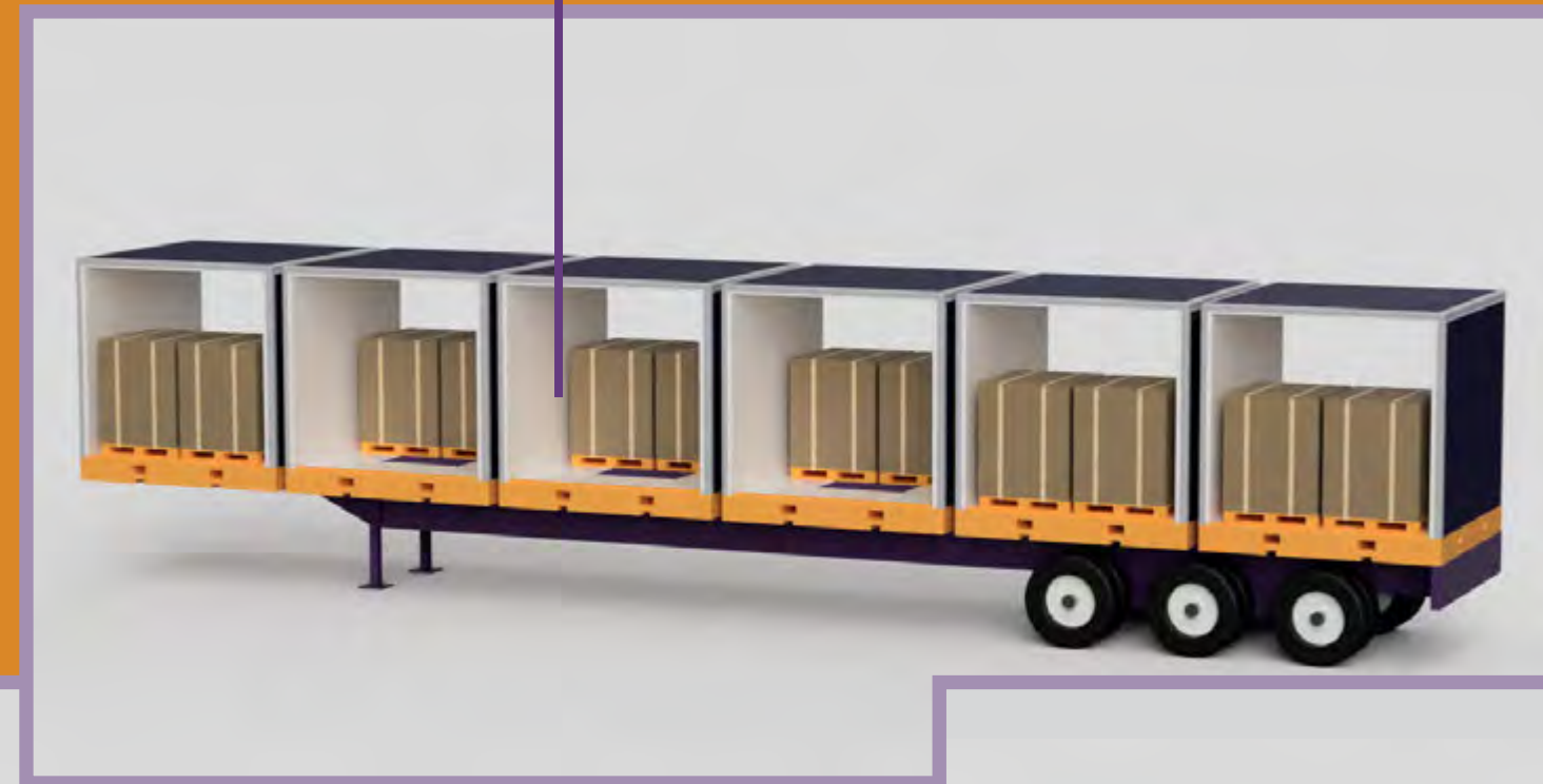
Delivery Mode - Doors are Outwards- facing on both sides.
